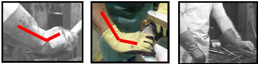
Pictures show wrist too bent and risky 1 hand pinching to lift heavy object.
